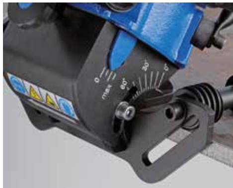
Seamless angle adjustment from 15° to 60°
