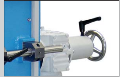
Axial adjustment of lower roll
