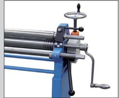
Drive with train of gear wheels and adjustment of back roll
