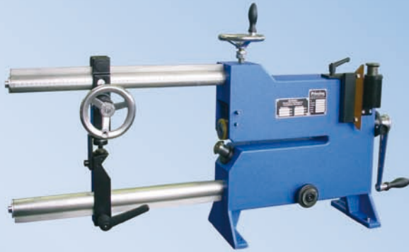
KS 10/10 With a flanging device* for external beading
